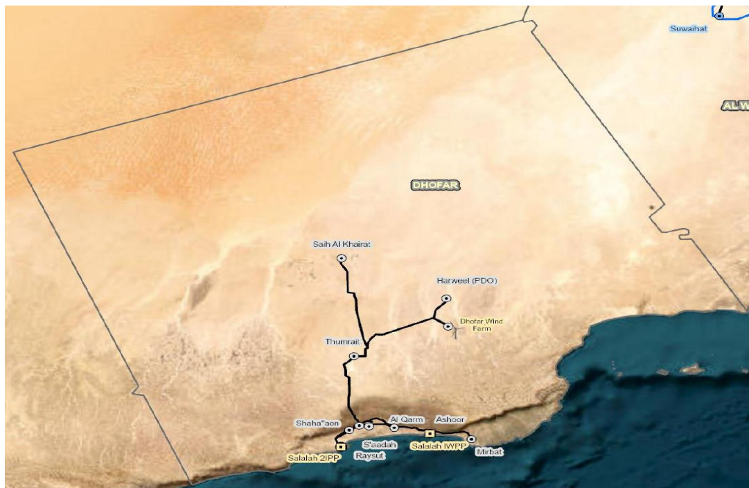
Figure 5.1-1 132 kV grid substations forming the regional transmission network in the Dhofar Region in the Y2025
